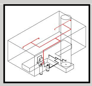
Standard-sized Down Draft - Booths using the ceiling as a plenum – The Amerex "IS" system has unique UL Listings that allow for options regarding the placement of nozzles. Nozzles may be placed in the traditional "H" pattern or they may be placed "Inline" down the center of the ceiling or even at the side walls. This allows nozzles to be placed out of the way for periodic replacement of the filters saving you time, money and hassle.
