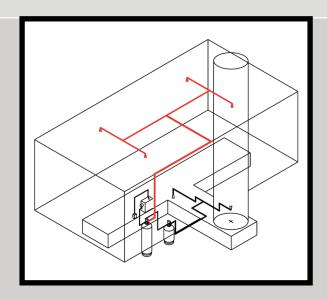
First Industrial system to be listed by UL under the newest edition of test Standard 1254 for nozzle heights up to 23'-4"above the floor – excellent for covering truck and heavy equipment spray booths.
